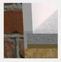
**2.** Add perimeter flanking strip to wall in preparation for SoundScreed being fitted.
