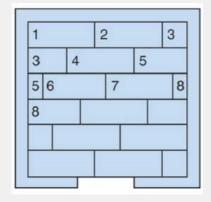
**6.** Use cut off from first row to start the next row. Lay the SoundScreed WF28 in a brick bond pattern butting up to the edging detail. (Minimum overlaps of 200mm)
